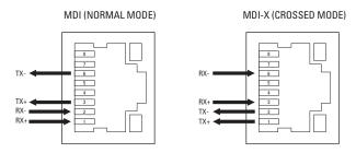
Figure 8. RJ-45 MDI/MDI-X Connector Pinouts
